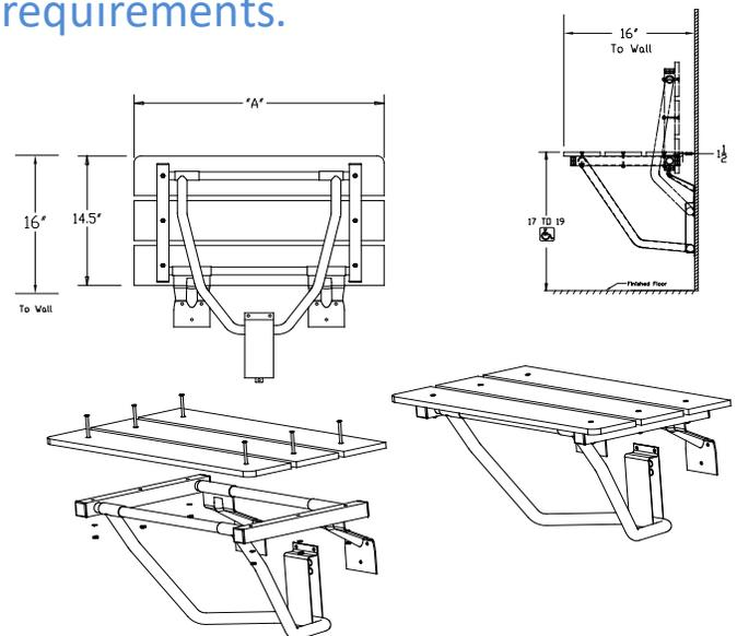
Elcoma Shower Seats have been designed and tested to withstand 400lbs. (182kgs) of load when properly installed.\* This exceeds HUD, FHA, VA, ADA, ANSI and other federal, provincial, and local codes. \*Shower seats can only be as strong as what they are mounted to. It is imperative when installing any shower seat to consult with a qualified contractor to insure you have sufficient backing.
