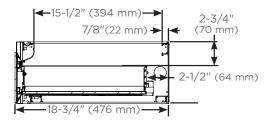
Side views for plumbing and sink clearance with door front
