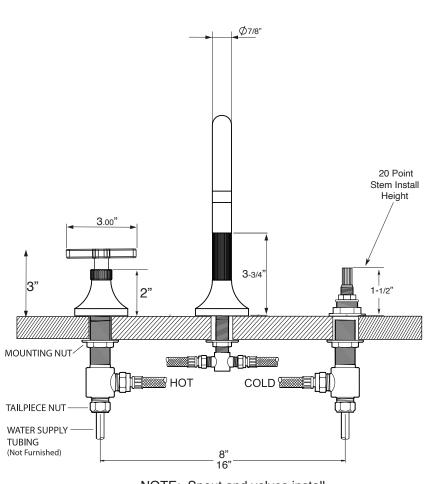
NOTE: Spout and valves install through 1-1/4" diameter holes
