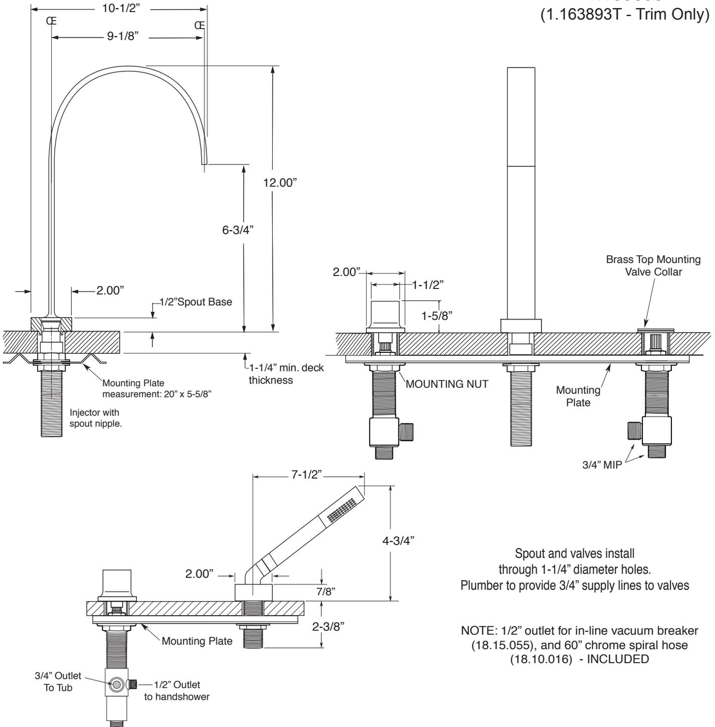
Spout and valves install through 1-1/4" diameter holes.
