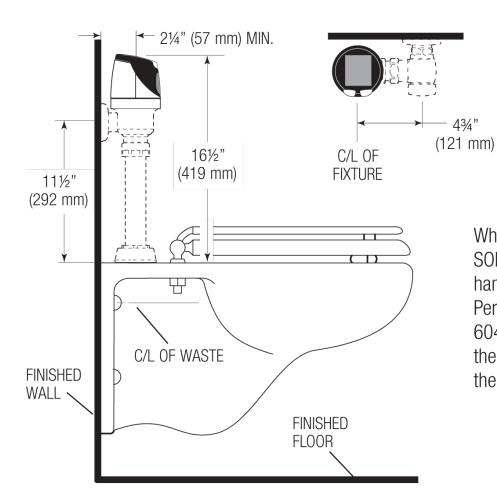
When installing the Sloan SOLIS™ Flushometer in a handicap stall: Per the ADA Guidelines (section 604.9.4) it is recommended that the grab bars be split or shifted to the wide side of the stall.
