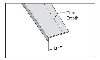
3. Measure, mark and cut the left and right vertical panels to the window jamb depth measurment (B).
