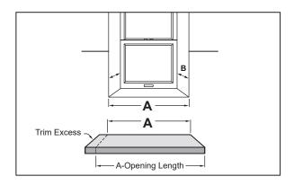
Measure, mark and cut the sill panel to the sill depth measurment (B). Trial fit the sill panel.Sand the cut edges with medium grit sand paper.
