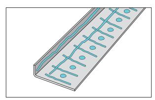
5. Apply silicone sealant to the underside of the sill panel as shown above. Install the sill panel, press down so the sealant makes good contact.
