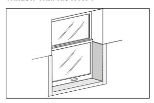
Measure the width (A) and depth (B) of the window opening. Trim the sill panel at the same width of the opening. (cut off the end with the factory holes, they are not used).
